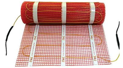
Installed into the tile adhesive, the standard 150W/m<sup>2</sup> mat heaters offer a faster warm up time when compared to in-screed & in-slab systems due to it's close proximity to the tile or stone floor surface.
